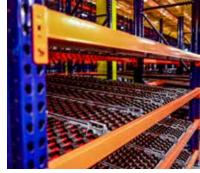
Well adapted for large distribution centers, they are constructed from basic pallet racking components. Sub-components consist of carton flow, pallet flow, various forms of shelving and conveyor, as well as flooring, handrails, stairs, kickplates, lighting, and fire sprinkler protection.
